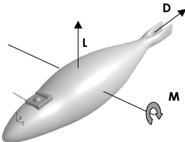
**Fig. 3** Lift, drag and pitching moment
